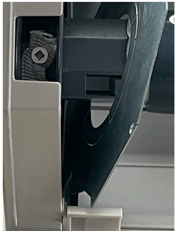
6.4 Screw the tape to the special hole in the plastic wheel
