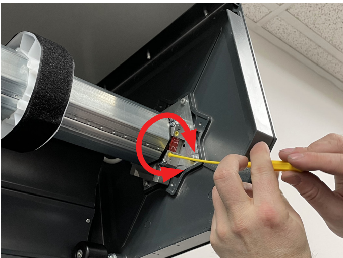
Use the bottom limit screw to lower the Curtain.
