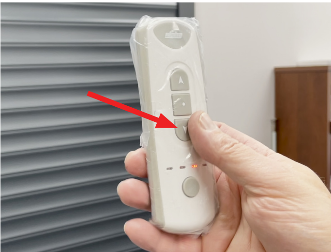
Use the remote to lower the curtain till it stops.
