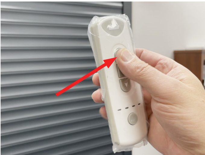
Use the remote to raise the curtain till it stops.
