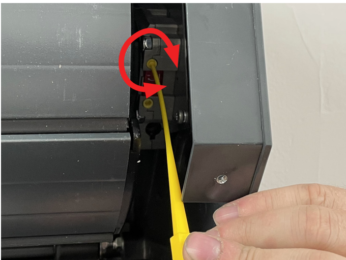
Use the upper limit screw to raise the Curtain.
